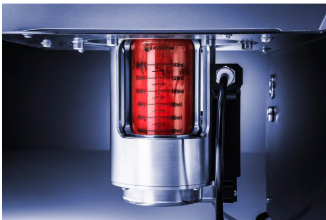
Figure 1: The powder flow cell mounted on a Modular Compact Rheometer (MCR) from Anton Paar.
